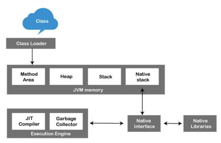
**ClassLoader:** ClassLoader is a subsystem used to load class files. ClassLoader first loads the Java code whenever we run it.
