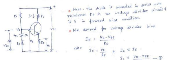
\* When VBE change with temperature Ic also changes. \* The voltage at the base VB is now
