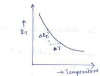
This method uses Temperature sensitive devices such as Thermistors rather than diode (or) Transiston \* It has negative temperature coefficient. its resistance decreases enponentially with increasin Temperature : as shown in fig:
