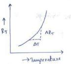
This method was temperature sensitive devices such as sensistor rather than diade (or) Transistor. \* It has a positive temperature coefficient. its resistance increases exponentially with increase temperature.
