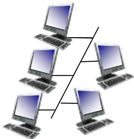
shared wire (e.g., cabled Ethernet)
