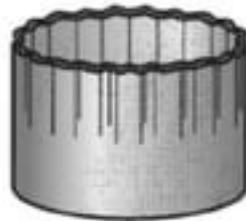
wrinkling in flange and cup wall
