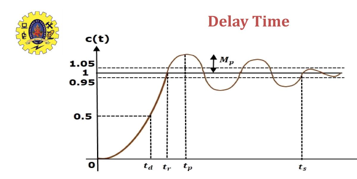
• It is the time required for the response to reach half of its final value from the zero instant. It is denoted by t<sub>d</sub> (sec)
