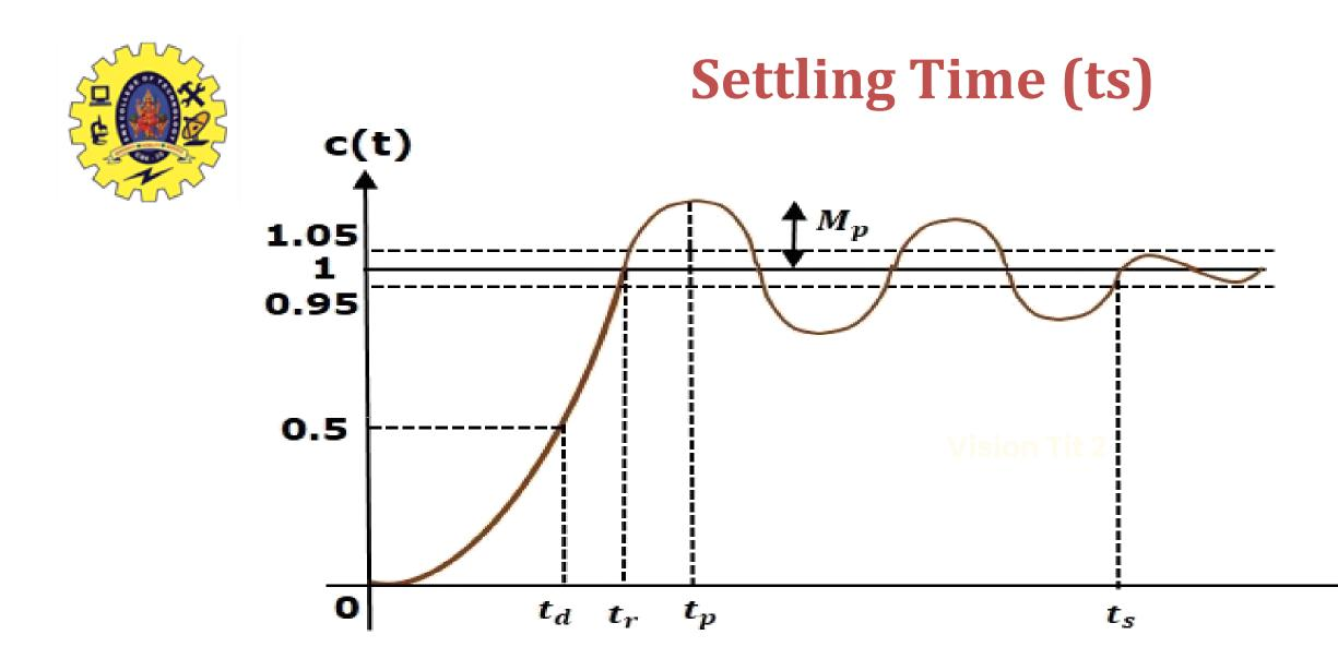
• It is the time required for the response to reach the steady state and stay within the specified tolerance bands around the final value. In general, the tolerance bands are 2% and 5%.
