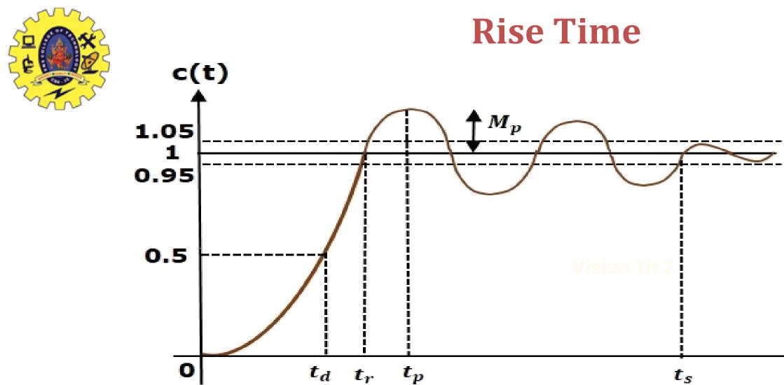
It is the time required for the response to rise from 0% to 100% of its final value and represented by t<sub>r</sub> (sec)
