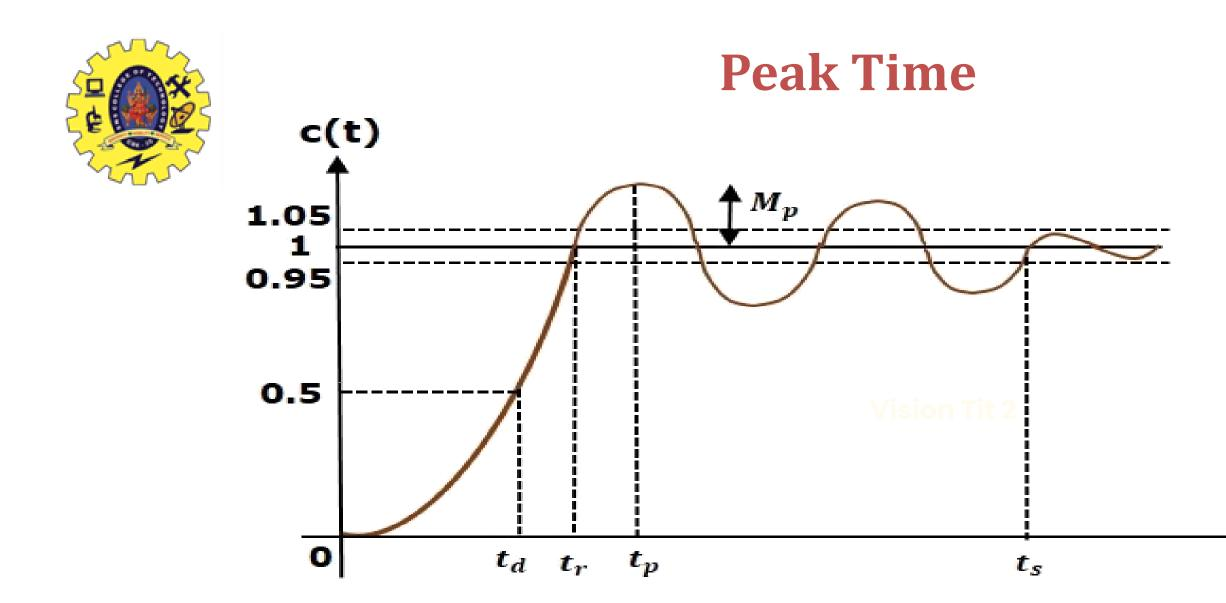
• It is the time required for the response to reach the peak value for the first time. It is denoted by  $t_p$  (sec). At t=t<sub>p</sub>, the first derivate of the response is zero.
