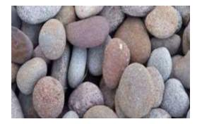
Irregular or partly rounded aggregates -Irregular aggregates may result 35- 37% of voids. These will give lesser workability when compared to rounded aggregates. The bond strength is slightly higher than rounded aggregates but not as required for high strength concrete.
