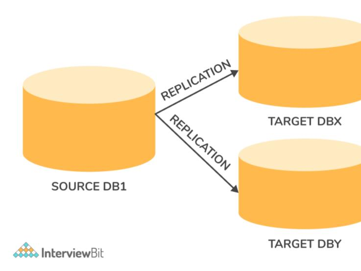
Replication of data is more than just a backup. A publisher is considered to be the server that originates the data, and a subscriber is the one where it is replicated. Data replication involves the publisher synchronizing its transaction with the subscriber and updating subscriber data automatically. A change made on the publisher's side is automatically reflected on the subscriber's side as well.
