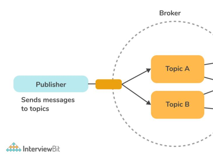
• **Push-Pull Model:** This communication model entails data producers pushing the data into queues, while data consumers pull the data from the queues. Neither producer nor consumer needs to know about each other. The queues help decouple the messages between the consumers and the producers. Also, queues act as a buffer when there is a mismatch between the rate at which producers push data and the rate at which consumers pull it.
