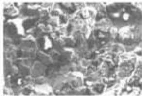
FIGURE 2.16 "Black matrix" porous surface of a grade 2 film marked by hydrogen evolution. (Courtesy of S. S. Fong, U.C.)
