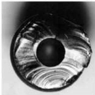
FIGURE 2.14 Track marks in a well track formed by debris (Courtesy of R. B. Peck, Jr.)
