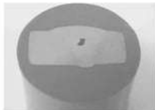
FIGURE 2.21 Clay inclusion in wall cover coating.
