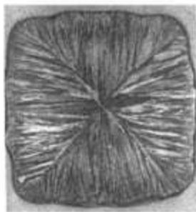
FIGURE 2.2 Agitation in cross section of carbon steel billet. (From Fundamentals and Applications, 1984, © 1976.)
