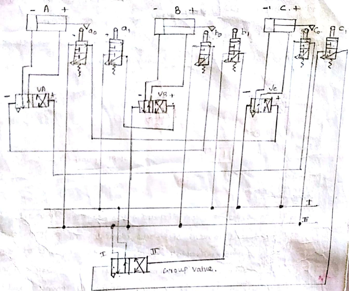
Cascade circuit for  $\frac{C}{\underline{A^+ B^+}} \frac{B^-}{\underline{T}} \frac{A^- C^+}{\underline{\Pi}}$
