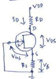
For dc analysis the coupling capacitors are replaced by open circuit &  $R_G$  is replaced by short circuit equivalent, since  $I_G = 0$ .
