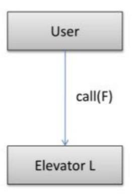
The user, inside the elevator L, user presses button to go to Floor F
