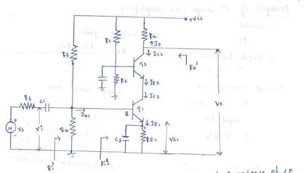
\* The Carcode amplifier gives The high isput inspedance of CE amplifier, as well as The good voltage gain 4 high frequency performance of CB circuit.
