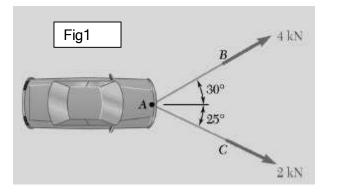
A disabled automobile is pulled by means of two ropes shown in fig 1. Determine the Magnitude and direction of Resultant by(a) parallelogram law,(b)Trianglelaw(c)analytical method
