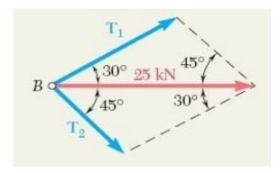
$T_1 = 18.5 \text{ kN}$   $T_2 = 12.8 \text{kN}$
