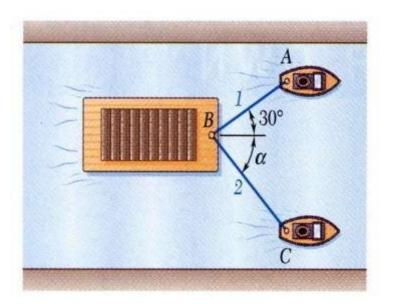
A barge is pulled by two tugboats. If the resultant of the forces exerted by the tugboats is a 25 kN directed along the axis of the barge, determine
