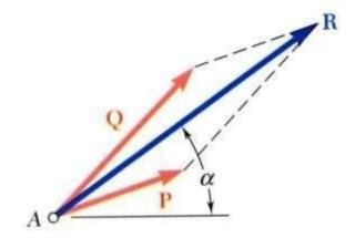
R Q P A • Graphical solution - A parallelogram withsides equal to **P** and **Q** is drawn to scale. The magnitude and direction of the resultant or of the diagonal to the parallelogram are measured,
