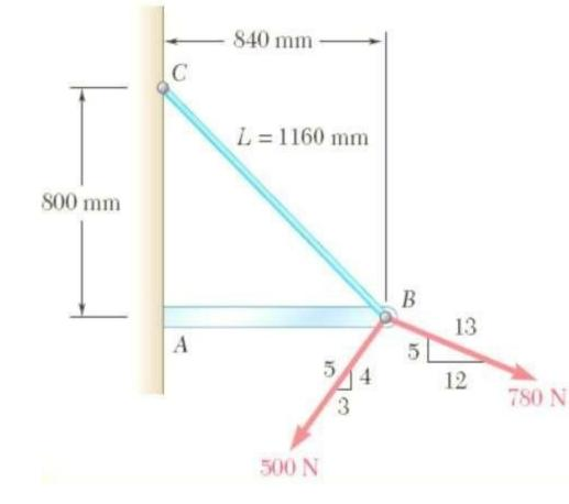
Knowing that the tension in cable *BC* is 725-N, determine the resultant of the three forces exerted at point *B* of beam *AB*.
