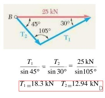
• Graphical solution - Parallelogram Rule with known resultant direction and magnitude, known directions for sides.
