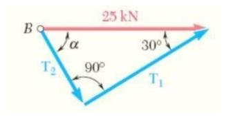
$T_2 = (25 \text{ kN}) \sin 30^\circ$   $T_2 = 12.5 \text{ kN}$
