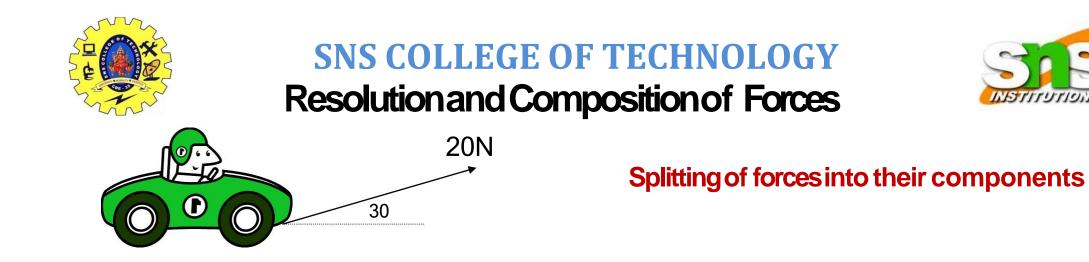
Resolution of force is a **reverse process** in which a singleforce is expressed in terms of its components. These components are sometimes referred to asthe resolved parts of the force.
