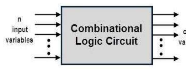
Combinational Logic Circuits are memoryless digital logic circuits whose output at any instant in time depends only on the combination of its inputs.
