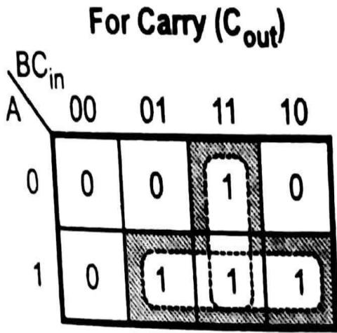
$$C_{out} = AB + A C_{in} + B C_{in}$$
