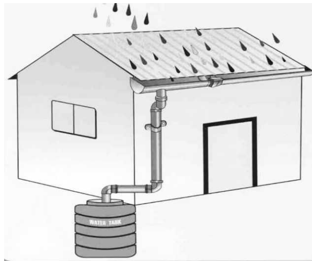
Fig. 1.10 Rooftop rainwater harvesting
