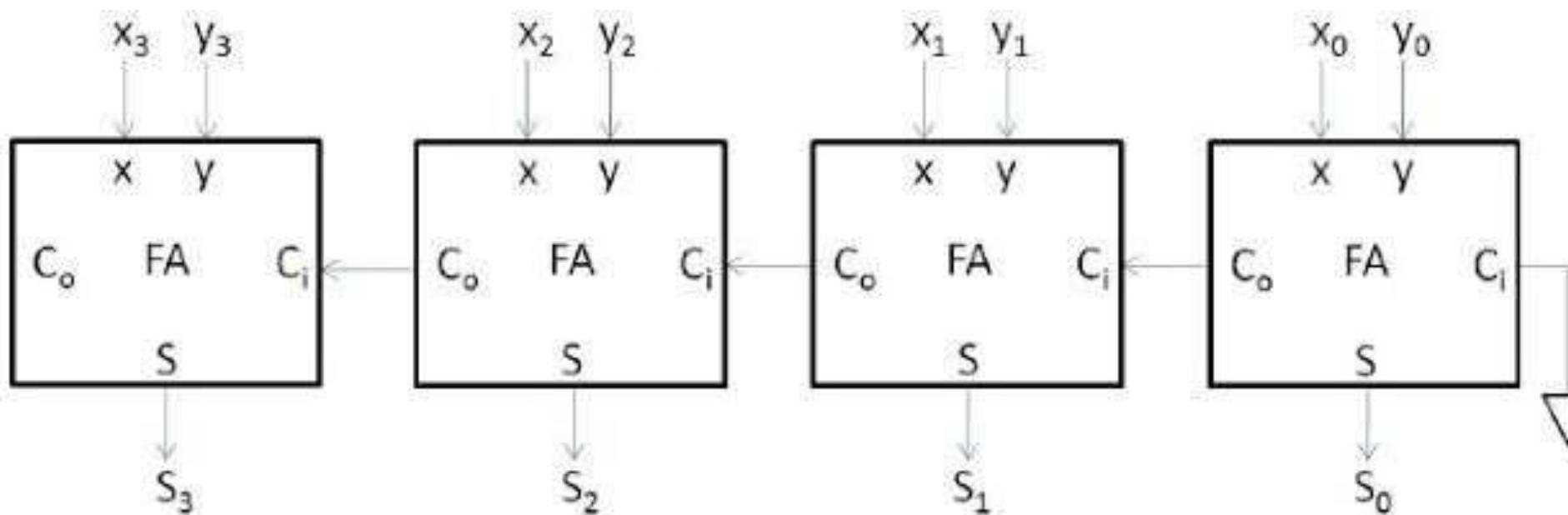
The 4-bit ripple-carry adder is built using 4 1-bit full adders
