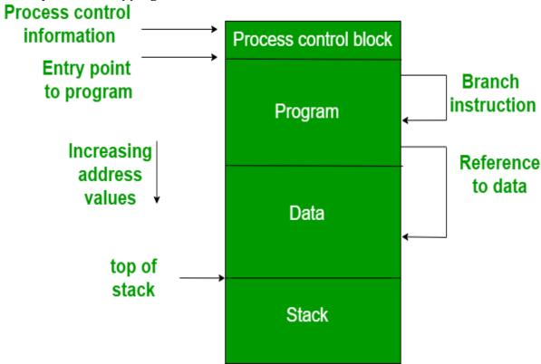
1. The figure depicts a process image. The process image is occupying a continuous region of main memory. The operating system will need to know many things including the location of process control information, the
