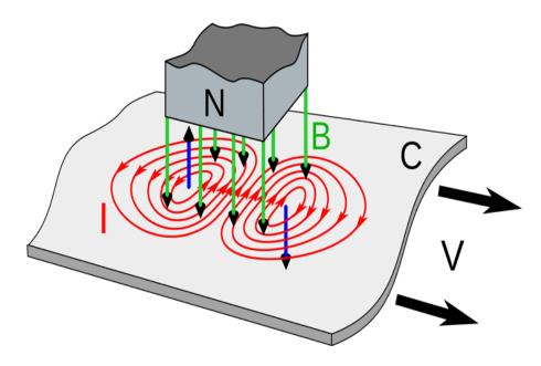
Eddy current (EC) testing is a no contact method for the inspection of metallic parts. Eddy currents are fields of alternating magnetic current that are created when an alternating electric current is passed through one or more coils in a probe assembly.
