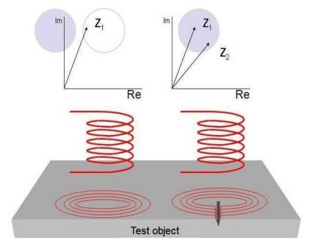
**Uses:** The technology is now widely used in the aerospace, automotive, petrochemical, and power generation industries for the detection of surface or near-surface defects in materials such as aluminum, stainless steel, copper, titanium, brass, Inconel®, and even carbon steel (surface defects only).
