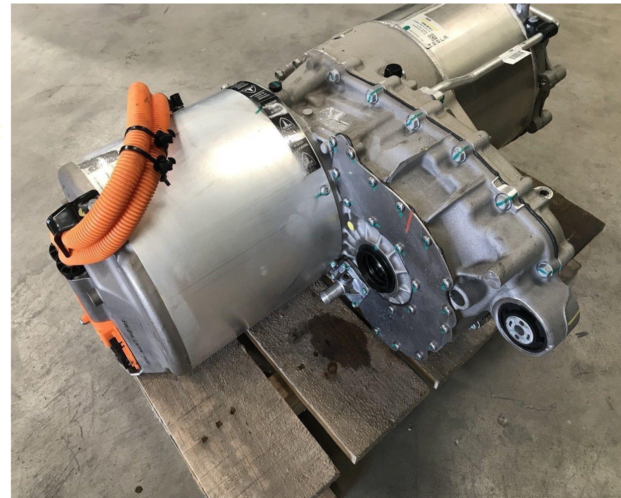
Tesla Model S Rear Drive Unit: The 3-phase 4-pole induction motor
