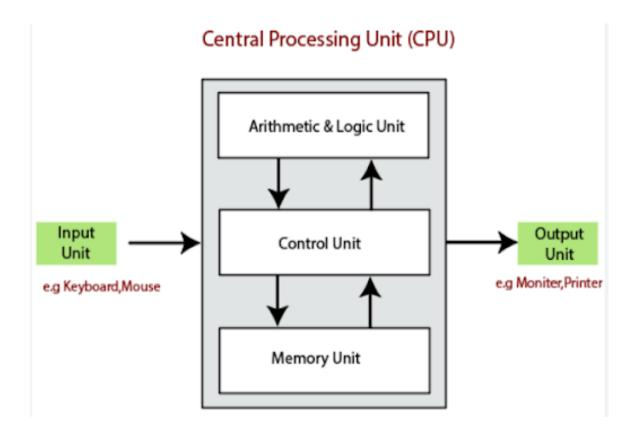
Block Diagram of a Computer helps us understand how a computer works, from collecting input data, processing & formatting the data, and generating the output results in the way user commands.
