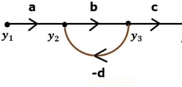
**Input Node** – It is a node, which has only outgoing branches. **Output Node** – It is a node, which has only incoming branches. segment which joins line Branch is a both gain and direction
