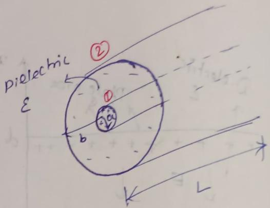
Coaxial cylindrical capacitor of length  $L$ .
