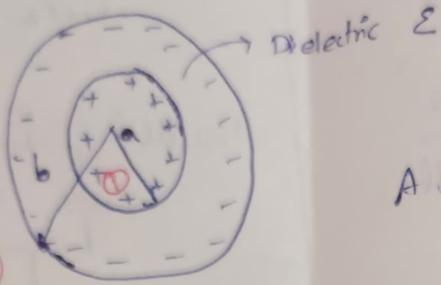
A spherical capacitor
