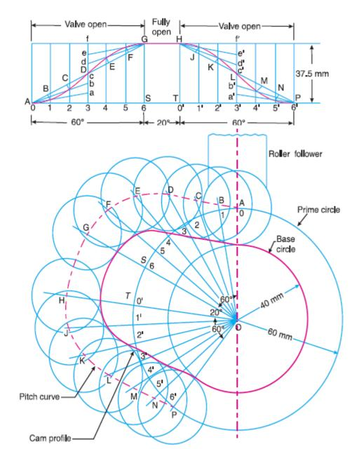
**Problem 5.** *Draw the profile of the cam when the roller follower moves with cycloidal motion during out stroke and return stroke, as given below:*
