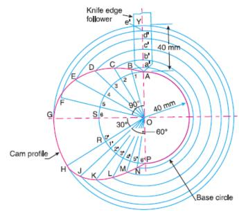
(b) Profile of the cam the cam when the line of stroke of the follower is offset 20 mm from the axis of the cam shaft
