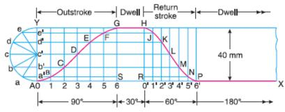
(a) Profile of the cam when the line of stroke of the follower passes through the axis of the cam shaft
