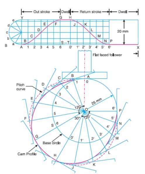
**Problem 4.** Design a cam for operating the exhaust value of an oil engine. It is required to give equal uniform acceleration and retardation during opening and closing of the value each of which corresponds to 60° of cam rotation. The value must remain in the fully open position for 20° of cam rotation.
