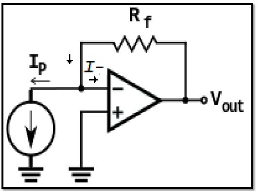
$\blacktriangleright$  A current to voltage converter will produce a voltage proportional to the given current.
