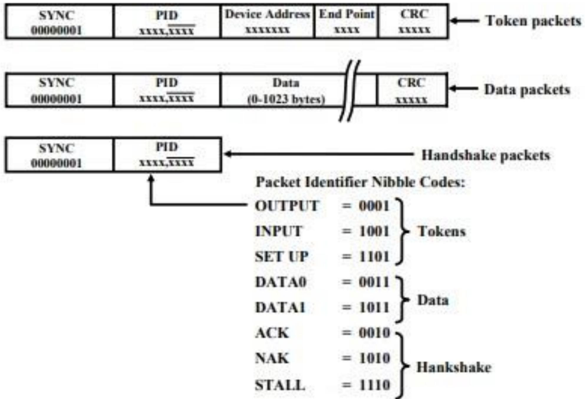
**Fig. 5 Examples of the various kinds of USB signaling and data packets.**
