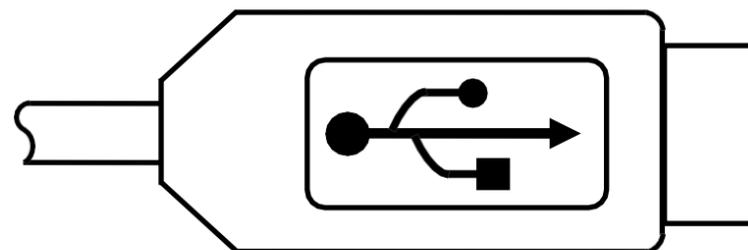
Fig. 4 Most USB plugs have this distinctive marking symbol.
