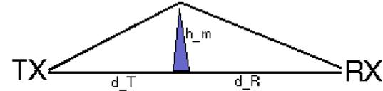
Fresnel zone: ellipsoid at which the excess path length is constant (e.g.  $\lambda/2$ )
