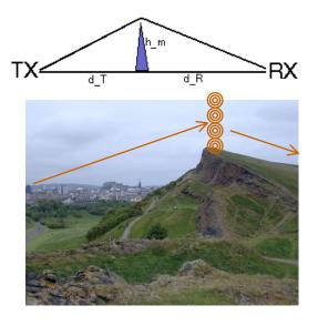
$h_m$  is the height of the obstacle, and  $d_t$  is distance transmitter - obstacle  $d_r$  is distance receiver - obstacle
