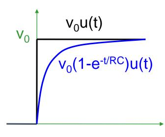
$$RC\frac{dv(t)}{dt} + v(t) = v_0 u(t)$$
