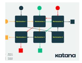
diagram depicting the flow of jobs through a series of workstations in a flow shop
