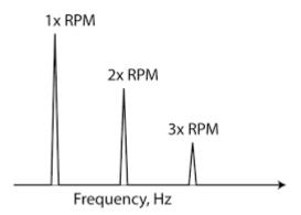
rotating machine with vibration sensors attached. The vibration data is collected and analyzed using Fast Fourier Transform (FFT) to identify characteristic frequencies associated with different faults.
