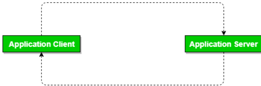
DBMS 2-Tier Architecture
