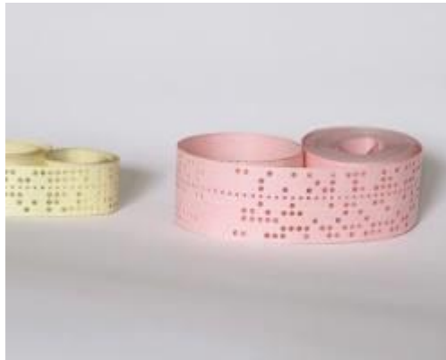
Punched Tape for Numerical Control
