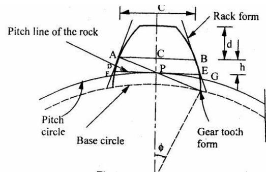
Vernier method like the chordal thickness and chordal addendum are dependent upon the number of teeth. Due to this for measuring large number of gears different calculations are to be made for each gear. So these difficulties are avoided by this constant chord method.
