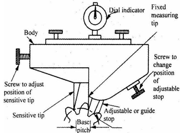
**Fig 3.16 Tooth to tooth measurement**
