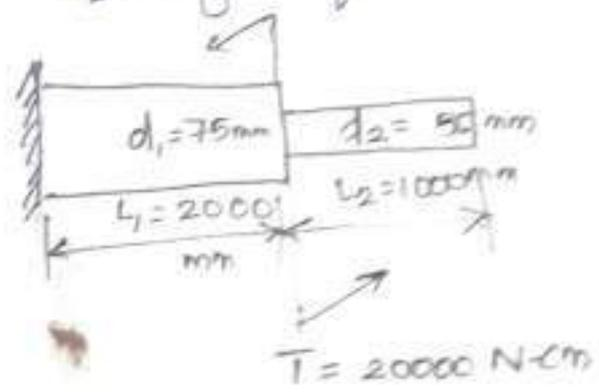
$$\frac{T}{J} = \frac{C\theta}{L} \quad \therefore T_1 + T_2 = 20000 \text{ N-m}$$
