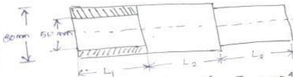
For shaft CD,  $J_3 = \frac{\pi}{32} D_3^4 = \frac{\pi}{32} \times 70^4 = 235.8 \times 10^4 \text{ mm}^4$
