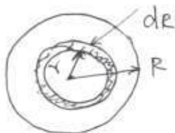
Turning force on elementary circular ring = (shear stress at)  $\times$  Area of ring
