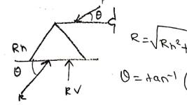
Roller Support has the known live of action or really an unknown live of action a reaction it and angle 0, with horizontar.
