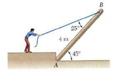
A man raises a 10 kg joist, of length 4 m, by pulling on a rope.
