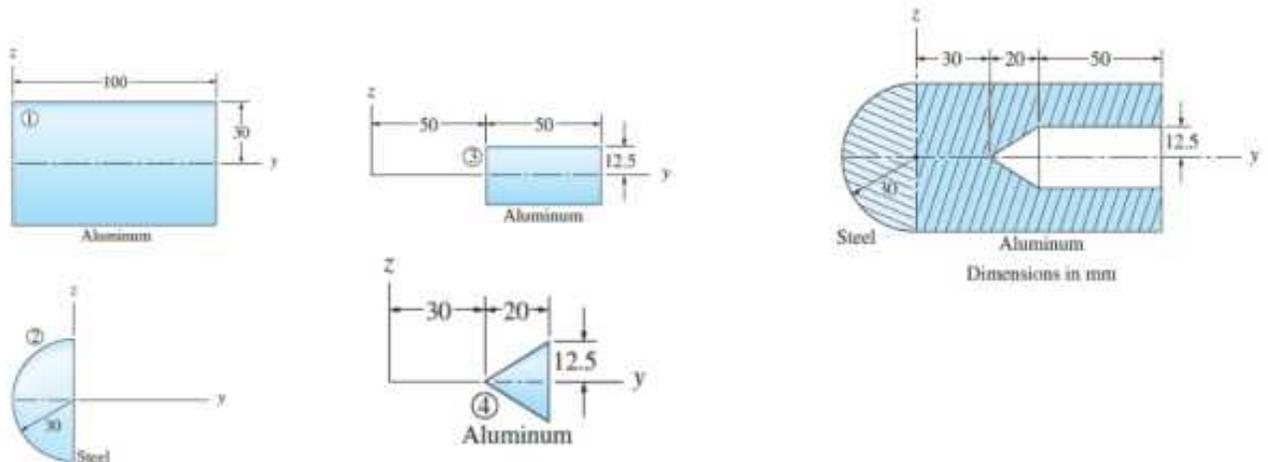
The part is composed of the four bodies shown in Fig. : the aluminum cylinder 1, plus the steel hemisphere 2, minus the aluminum cylinder 3, minus the aluminum cone 4. Because each of these bodies is homogeneous, each center of mass coincides with the centroid of the enclosing volume.
