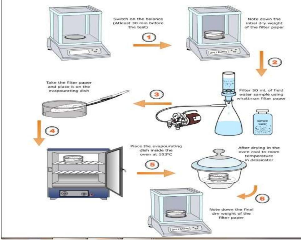
Suspended Solid (mg/L) = [(W<sub>2</sub>-W<sub>1</sub>) x 1000] / volume of sample Where:
