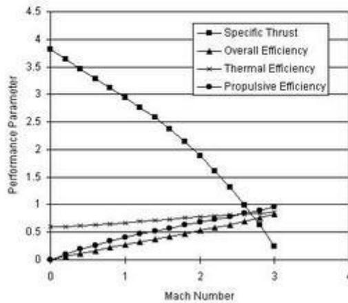
Performance of an ideal turbojet engine as a function of flight Mach number.
