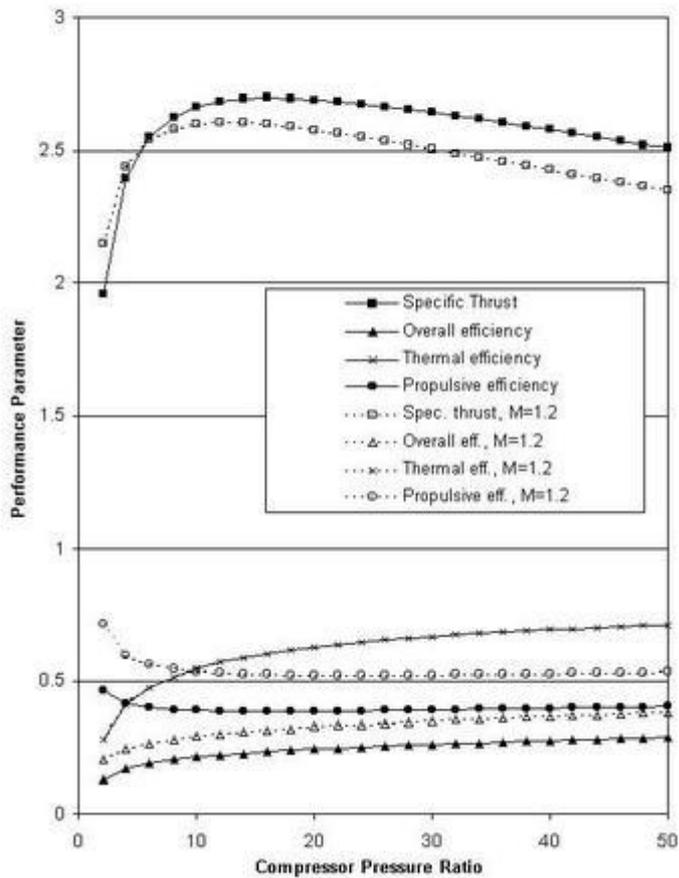
Performance of an ideal turbojet engine as a function of compressor pressure ratio and flight Mach number.
