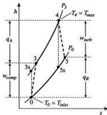
Gas turbine engine (Brayton) cycle showing the effect of departure from ideal behavior in compressor and turbine
