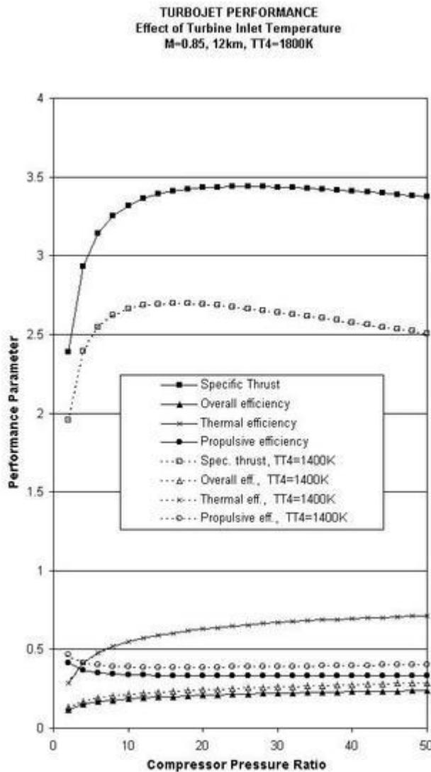
Performance of an ideal turbojet engine as a function of compressor pressure ratio and turbine inlet temperature.
