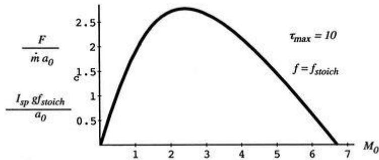
Thrust per unit mass flow and specific impulse for ideal ramjet with stoichiometric combustion [Kerrebrock]
