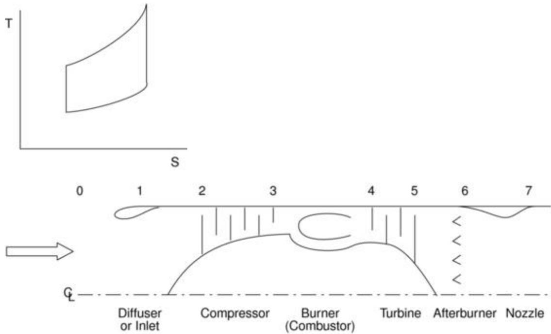
Gas turbine engine station numbering.
