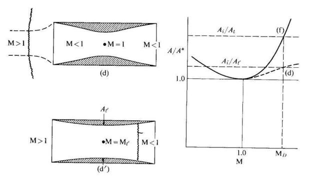
An inlet having  $A_i/A_t$  greater than 1 ( $A_i>A_t$ ) will always require spillage upon reaching supersonic flight velocities since Aa/At will always pass through a minimum of 1 just as sonic flight velocity is attained. It is necessary to perform some operation other than simply accelerating to the design speed to "swallow" the starting shock and establish isentropic flow. Overspeeding is one such operation, but there are others.
