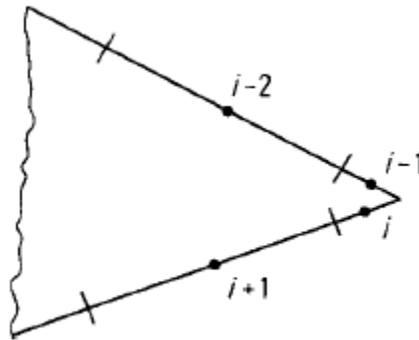
**Figure 1.11 Vortex panel at the trailing edge**
