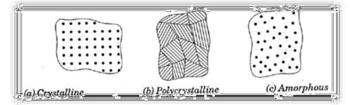
Difference between crystalline and amorphous material.
