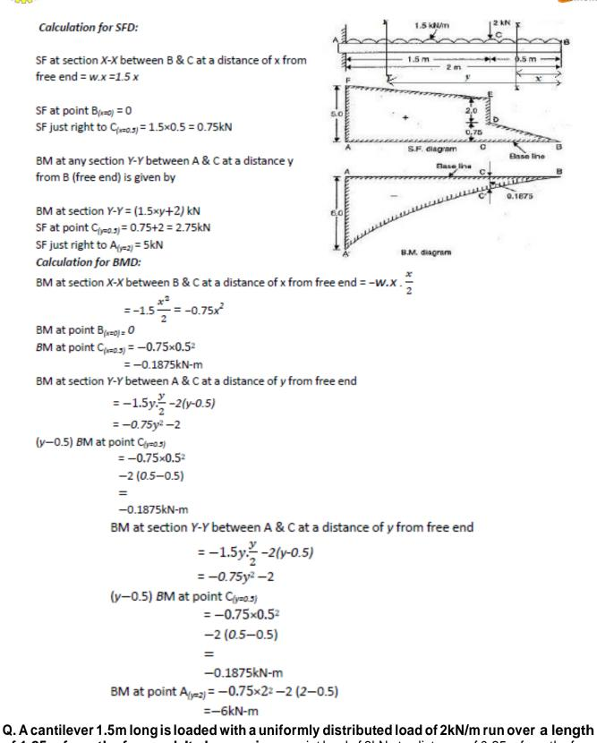
of 1.25m from the free end. It also carries a point load of 3kN at a distance of 0.25m from the free end. Draw SFD & BMD of cantilever.
