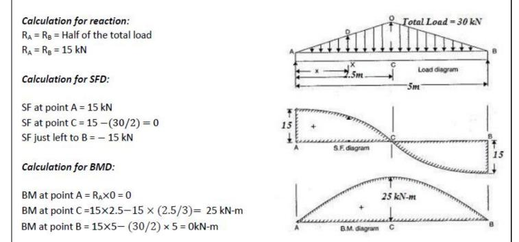
Simply Supported beam with a gradually varying load from zero at one end to w per unit length at other end
