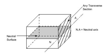
We know that when a beam is under bending the fibres at the top will be lengthened while at the bottom will be shortened provided the bending moment M acts at the ends. In between these there are some fibres which remain unchanged in length that is they are not strained, that is they do not carry any stress. The plane containing such fibres is called neutral surface.
