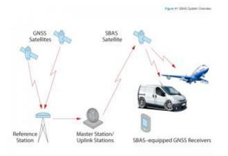
Corrections are uplinked to the SBAS satellite then broadcast to GNSS receivers throughout the SBAS coverage area. User equipment receives the corrections and applies them to range calculations. The following sections provide an overview of some of the SBAS services that have been implemented around the world or that are planned.
