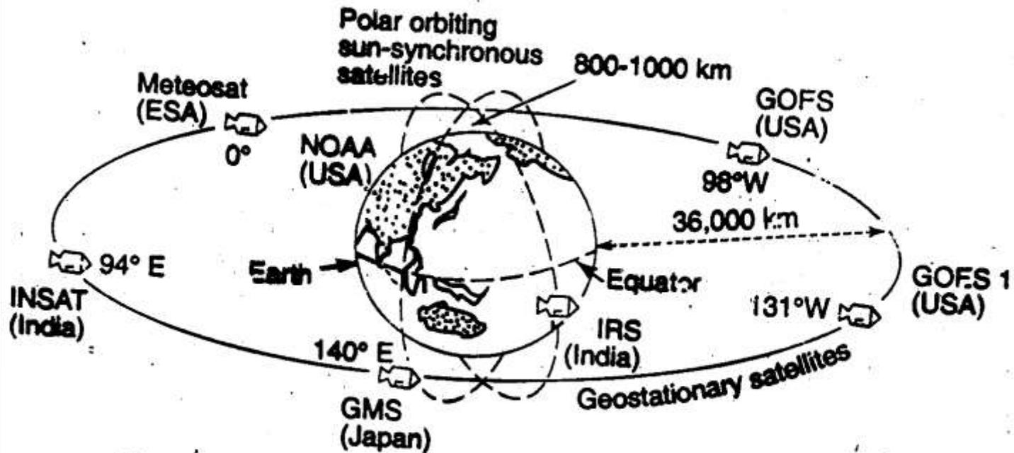
**Fig. 2.5** Geostationary and sun-synchronous satellites
