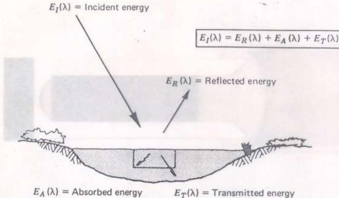
**FIGURE I.6** Basic interactions between electromagnetic energy and an earth surface feature.
