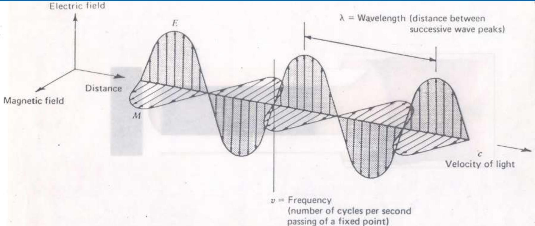
**FIGURE I.2** An electromagnetic wave. Components include a sinusoidal electric wave ( $E$ ) and a similar magnetic wave ( $M$ ) at right angles, both being perpendicular to the direction of propagation.
