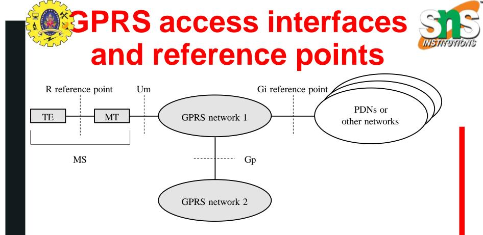
PRS provides packet switched connections from MS to acket data networks (PDN)
