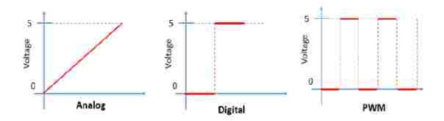
Difference between Analog, Digital and PWM Pins
