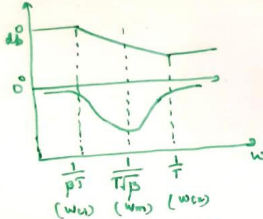
$$\omega_m = \sqrt{\omega_{c1} \omega_{c2}} = \sqrt{\frac{1}{\beta T} \cdot \frac{1}{T}} = \frac{1}{T\sqrt{\beta}}$$
