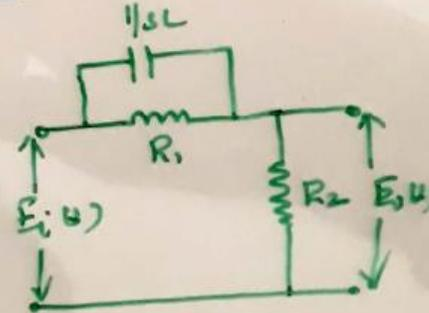
$$\frac{E_o(s)}{E_i(s)} = \frac{s + \frac{1}{R_1C}}{s + \frac{1}{R_2C}}$$
